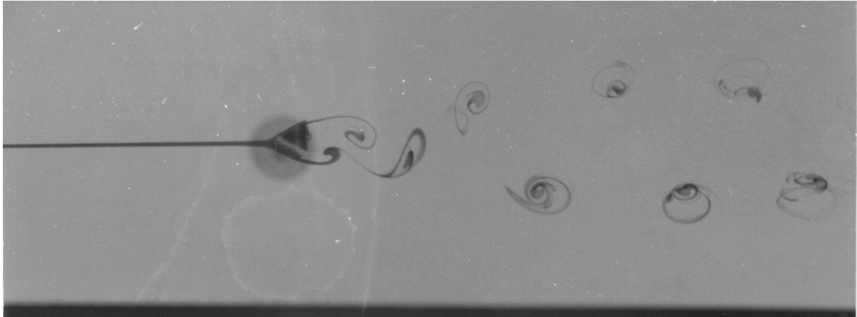
Figure 3 Wake generated by a triangular cylinder - Reynolds number about 200.
